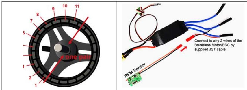
3. Long pressing the Key until the RED LED Soiled ON to enter Pole Pairs setting mode. Set the number on the RPM sensor by push the key repeatedly until you've got the correct number (**The Digital number is Binary value, see below chart for details**). Power off the receiver after set.
